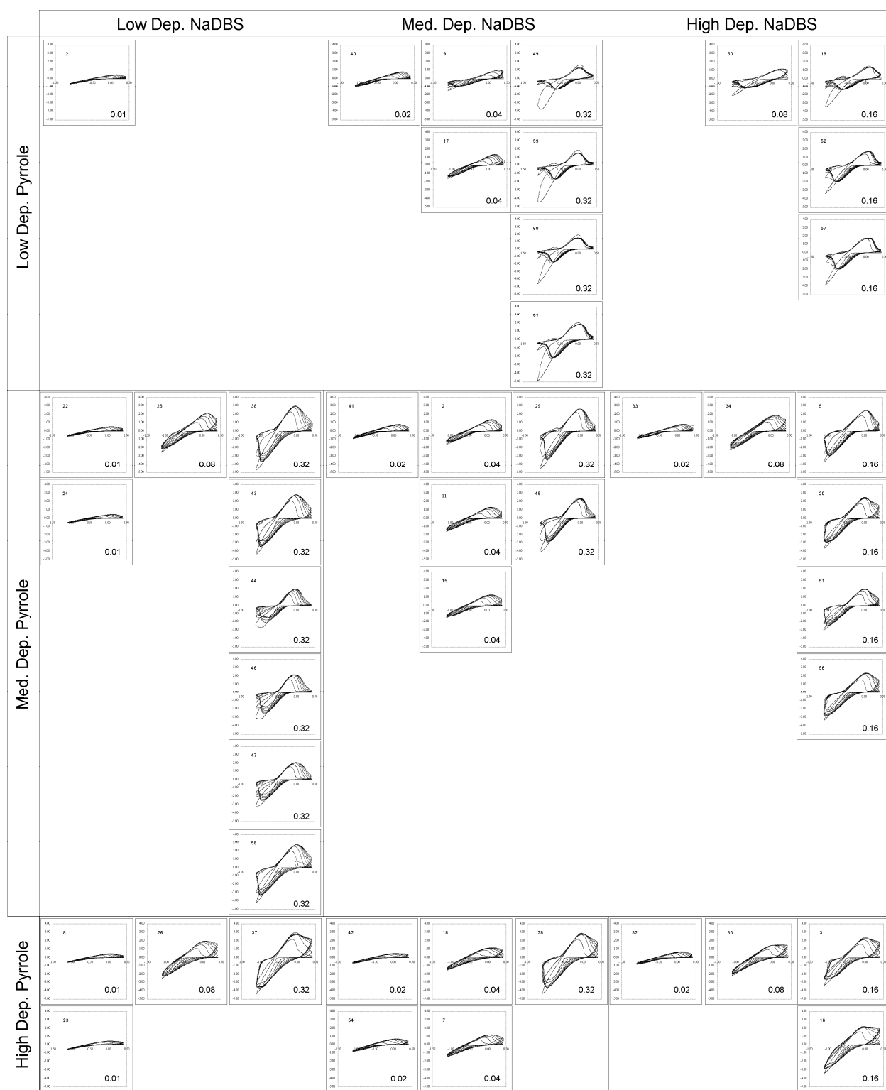
Fig.-SM 3. Cyclic voltammograms grouped by NaDBS concentration (columns), pyrrole concentration (rows), and stimulation NaDBS concentration (columns within columns). All y-axes are from -5 to 4 mA, and x-axes are from -1.5 to +0.5 V vs. Ag/AgCl. Labels on the lower right of each CV indicate the cycling NaDBS concentration, on the upper left the sample number.
